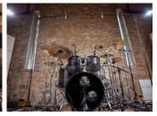
Again, two KM 184 small-diaphragm microphones are used as overheads. The video shows that instead of an XY setup, an AB constellation (time-of-arrival difference instead of level difference) can also be useful here. On the snare, a Neumann KMS 105 is used, which was designed as a high-quality stage vocal microphone, but works very well on the snare drum, too, while suppressing the hi-hat due to its supercardioid pickup pattern.
