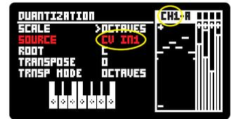
CHANNEL 1 QUANTIZING CV INPUT 1 VOLTAGE
