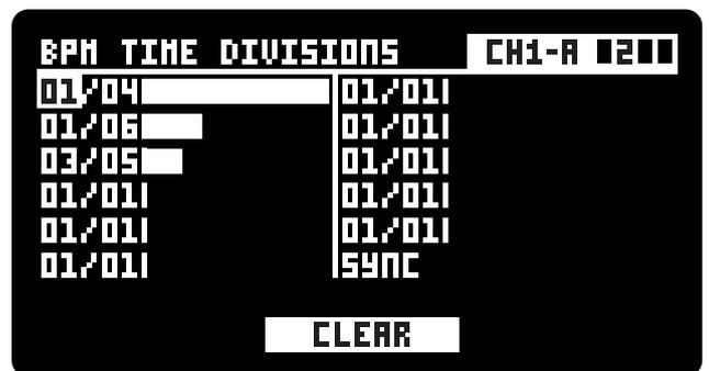
The SYNC slot output division is variable, it outputs the required time until the next beat. This will make sure the next step falls back on the beat. This is especially usefull when using odd time divisions as it resets any offset, you can see a graphical example below.
