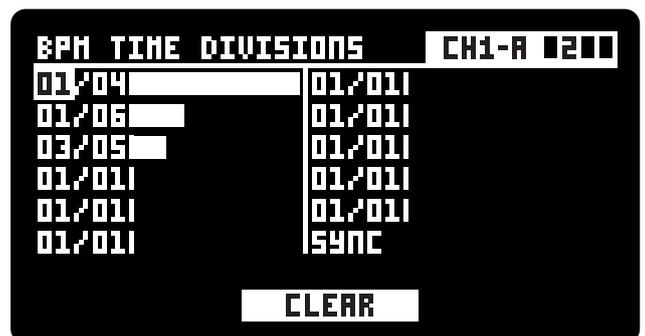
The SYNC slot output division is variable, it outputs the required time until the next beat. This will make sure the next step falls back on the beat. This is especially useful when using odd time divisions as it resets any offset, you can see a graphical example below.
