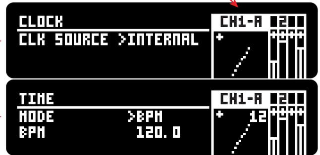
Channel 2 [CLK SOURCE] is set to sync to Channel 1
