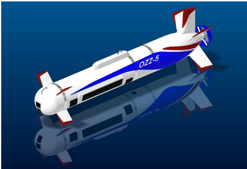
OZZ-5, autonomous underwater mine countermeasure detection vehicle © Mitsubishi Heavy Industries
