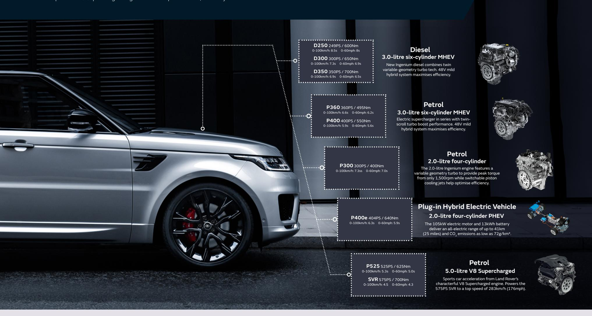
State-of-the-art new six-cylinder diesel engine features a 48V mild hybrid system to harvest energy normally lost during deceleration and intelligently redeploy it to assist the engine and maximise efficiency. Additional benefits include;
