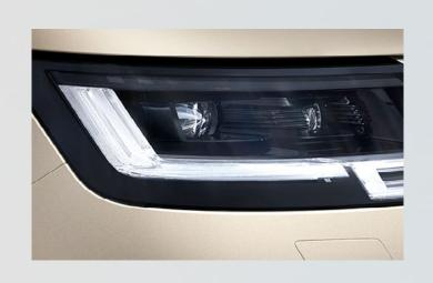
Digital LED headlights with industry leading microprocessor and 1.2 million micromirrors, can focus on 16 objects simultaneously and blank out reflections.
