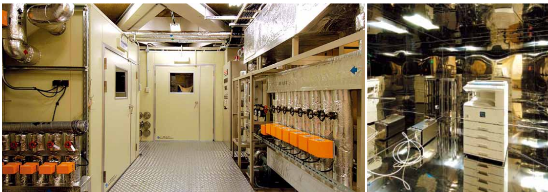
Emission-measuring testing laboratory (Ricoh Ohmori office)
