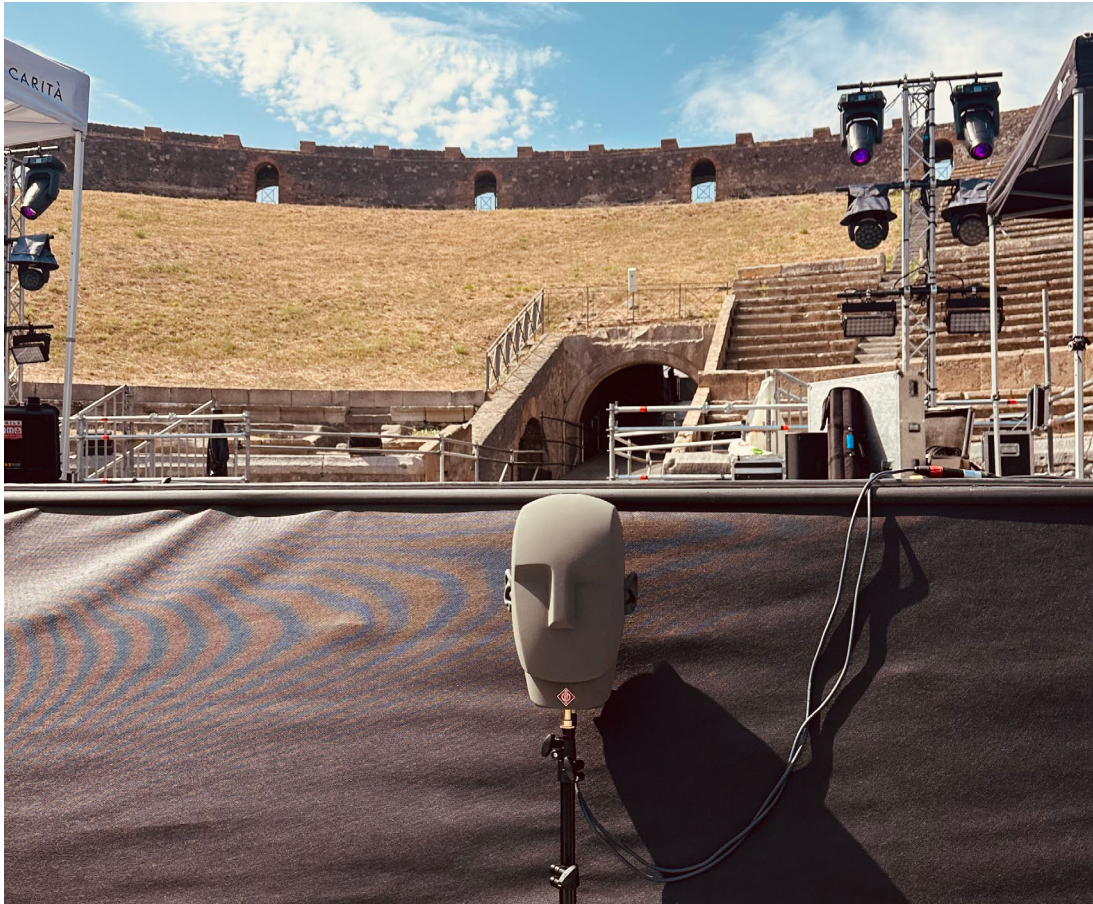
A Neumann KU 100 binaural head serves to capture the concert so Bryan Adams can listen back from the audience perspective. On larger shows with in-ears, it is also used for the monitor mix. Photo: Stefan Holtz
