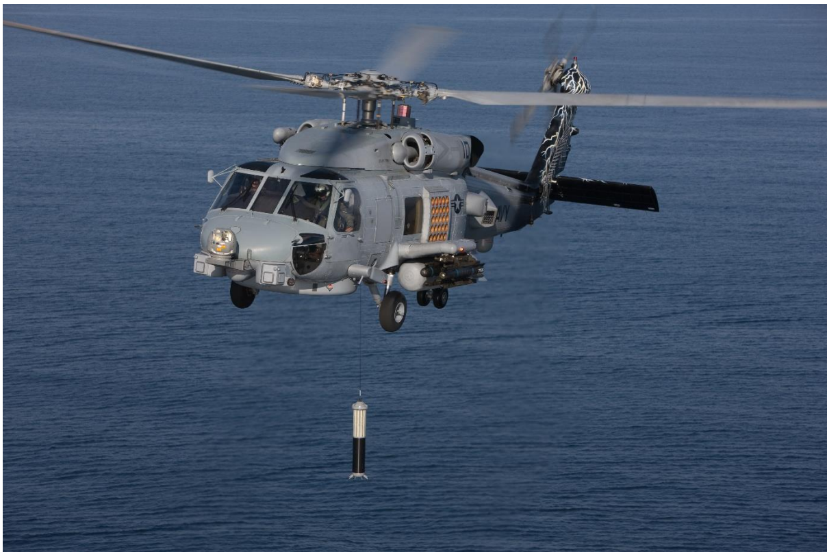
ALFS dipping sonar on MH-60R helicopter © Lockheed Martin
