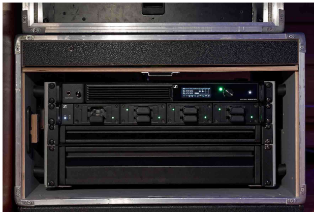
Space-saving: the Spectera Base Station with an L 6000 charging unit
