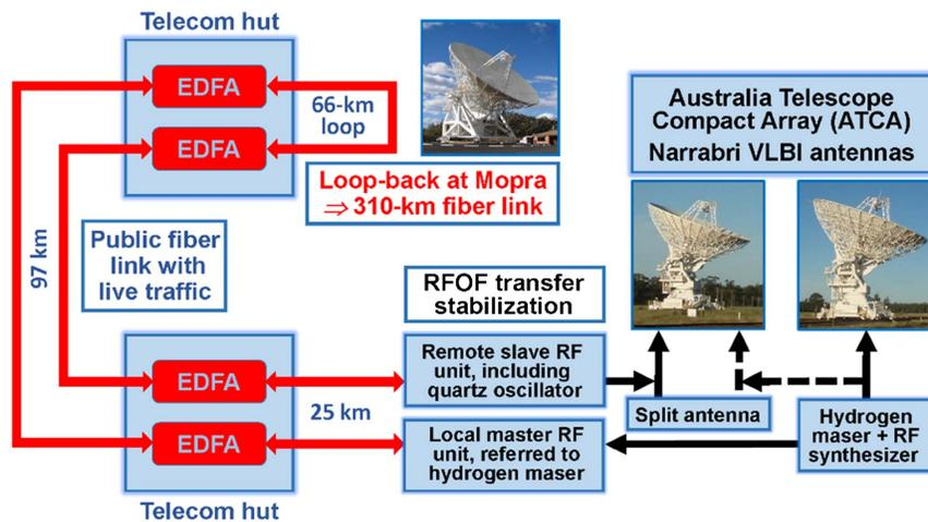
**Fig. 3.** RFOF loop-back transfer configurations for phase-stability experiments. The RF reference derived from a hydrogen maser at ATCA (Narrabri) is sent to Mopra and looped back to ATCA over a 310-km fiber link (red double-ended arrows). Configurations for the master and slave RF references are shown as black single-headed arrows (dashed for extra connections to the second path of the split antenna).
