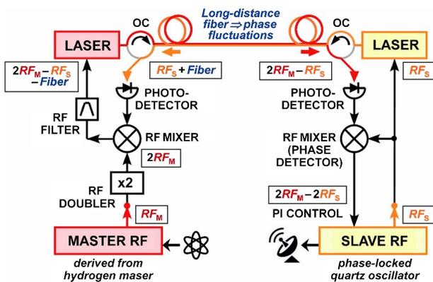
F1:1 **Fig. 1.** RFOF transfer schematic. The local (master) and remote (slave)
