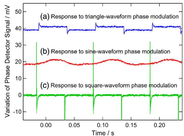
**Fig. 7.** Impact on RFOF transfer of phase fluctuations in the input RF reference. Responses of the RFOF phase detector to (a) triangle, (b) sine, and (c) square waveforms’ phase fluctuations in  $RF_M$  and identical  $RF_S$  using 50 km of spooled fiber. Phase fluctuations in three different forms were simulated by using a signal generator.
